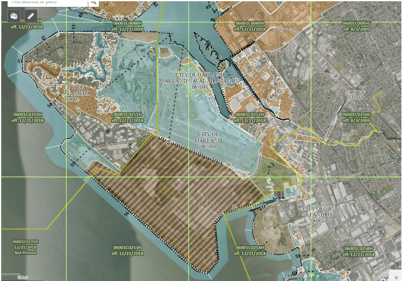
Figure 5-12. FEMA Flood Zones for Bay Farm Island
