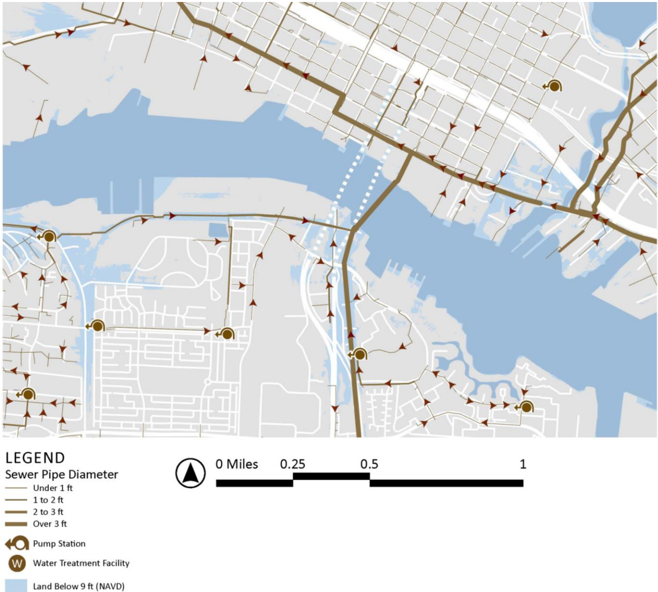
Figure 4-2424. Sewage System Surrounding Oakland-Alameda Estuary
