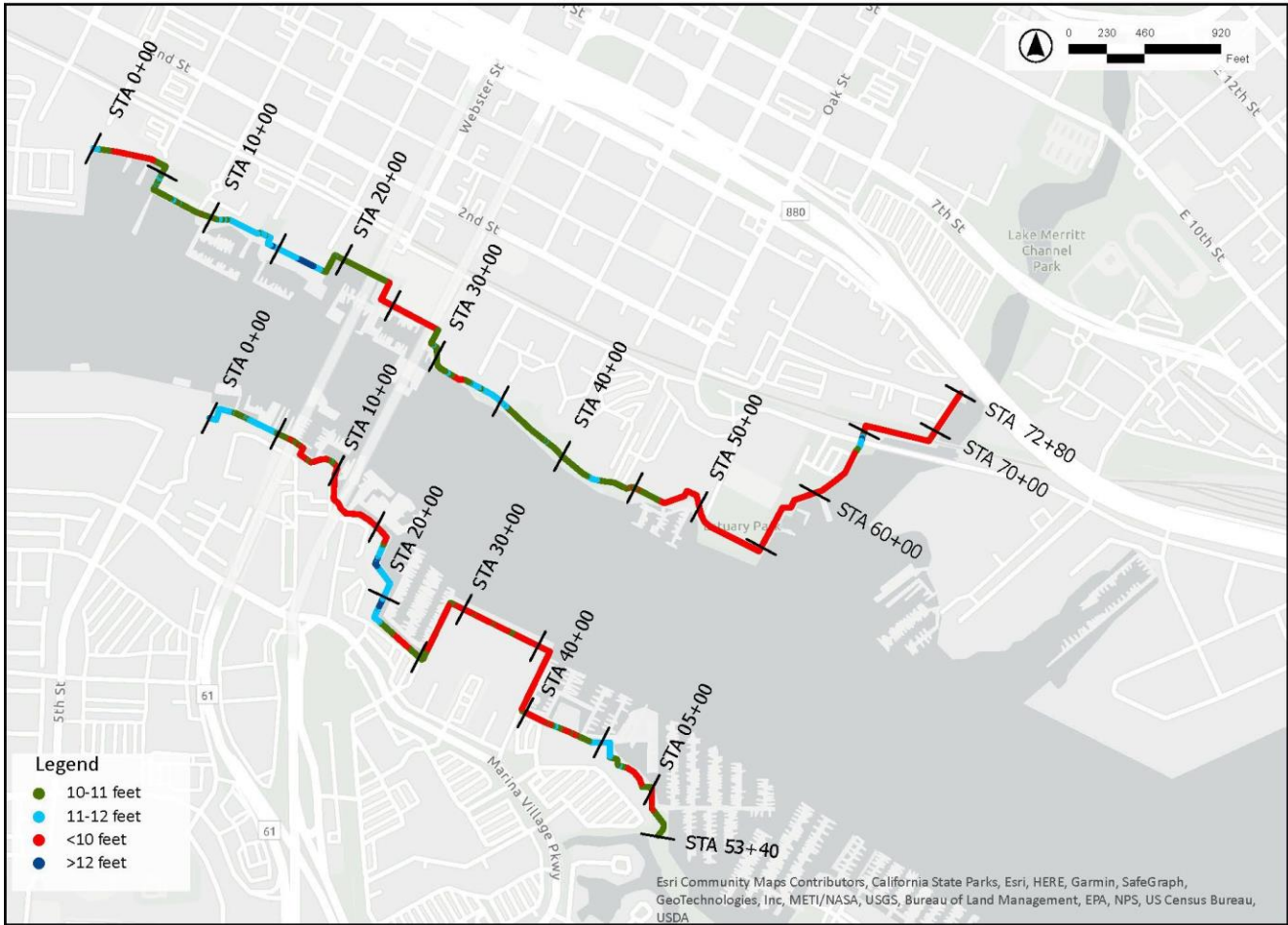
Figure 4-17. Oakland Shoreline Elevations – Plan View
