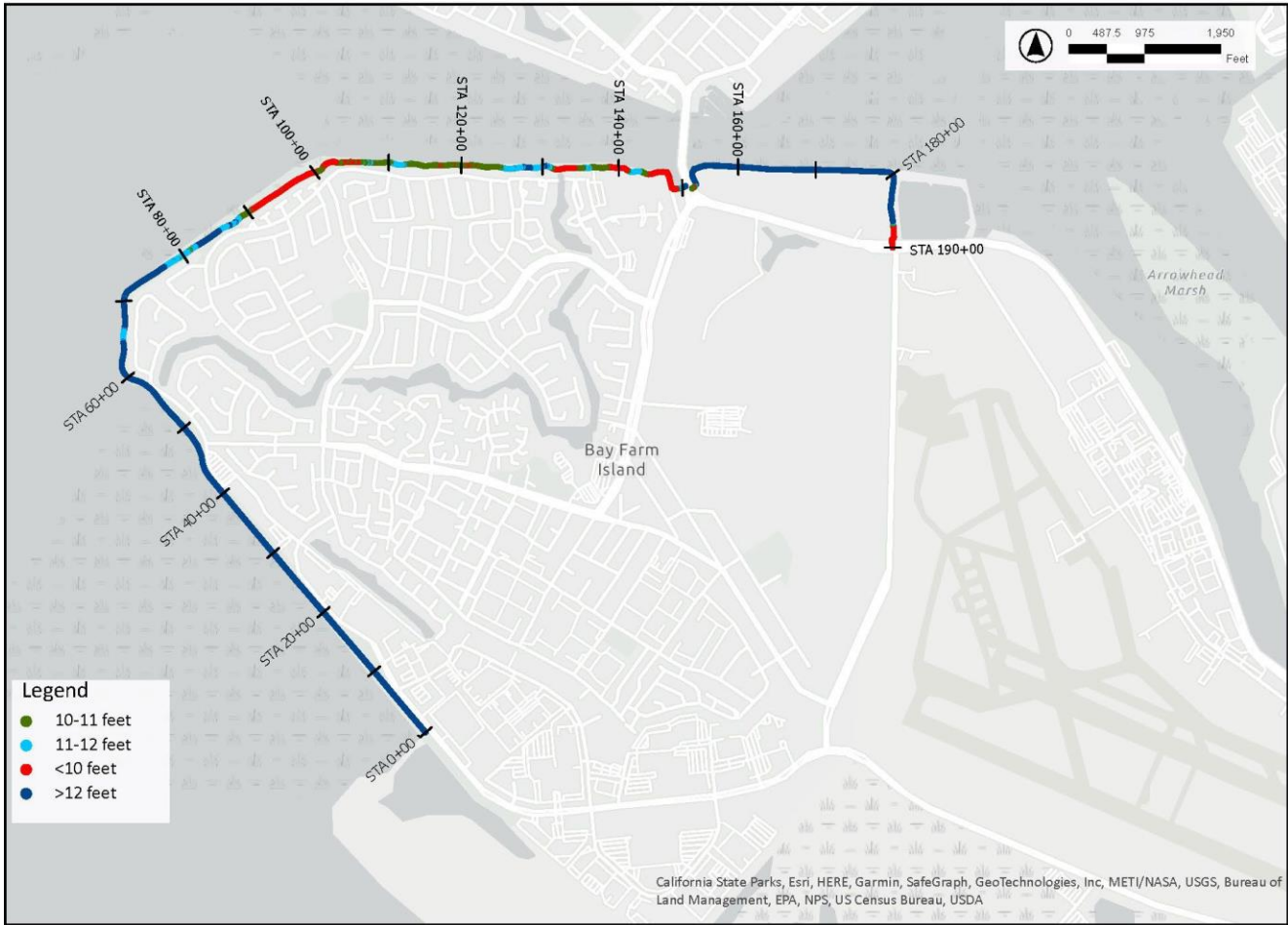
Figure 5-23. Bay Farm Island Shoreline Elevations – Plan View
