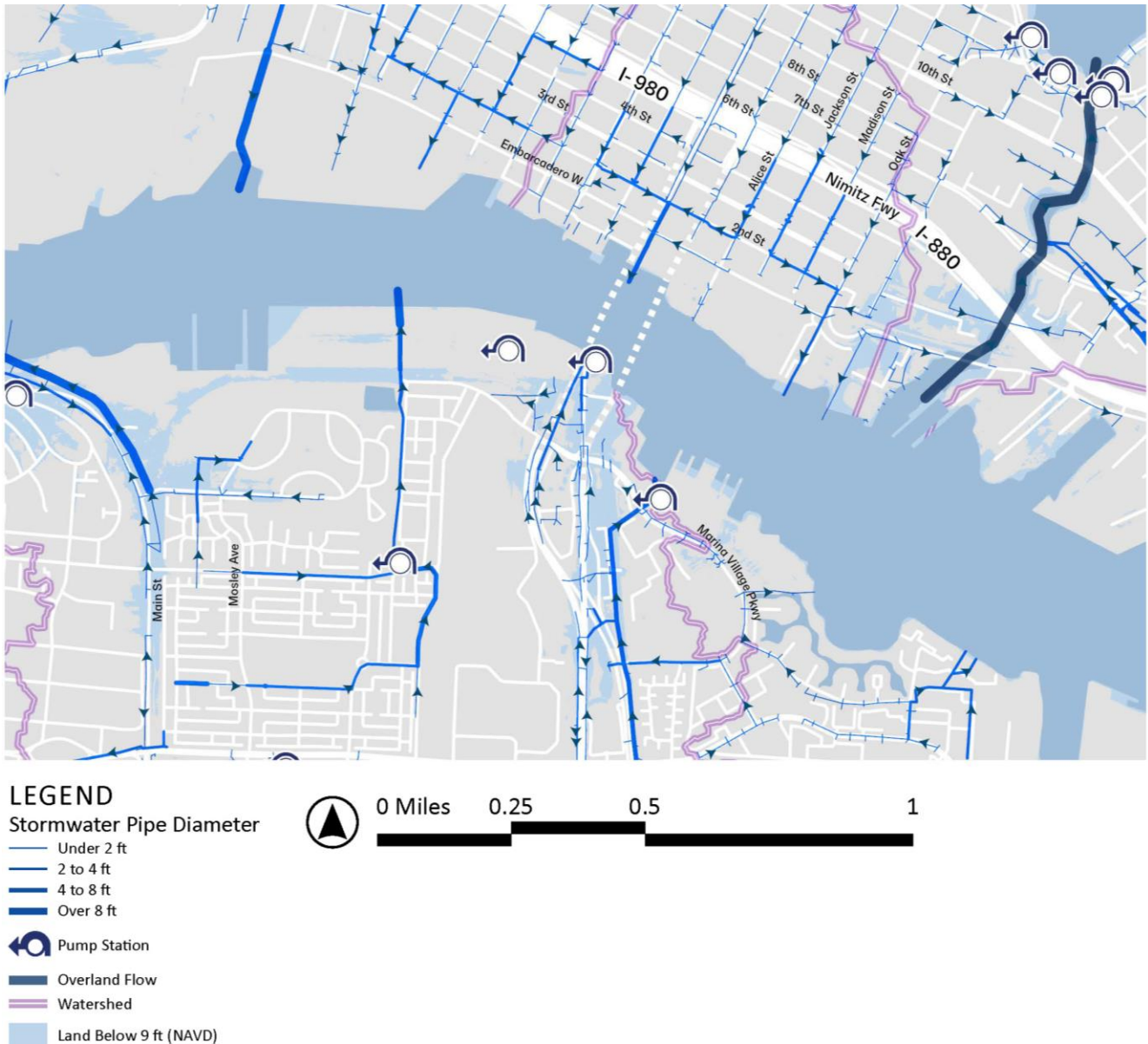
Figure 4-2323. Storm Drain Network surrounding Oakland-Alameda Estuary
