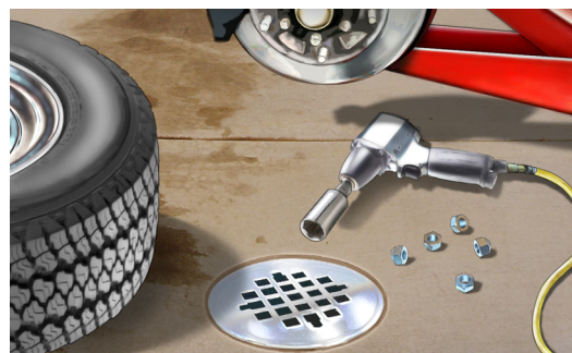
Sanitary Sewer Drain: An indoor drain that flows to the Sewage Treatment Plant.
