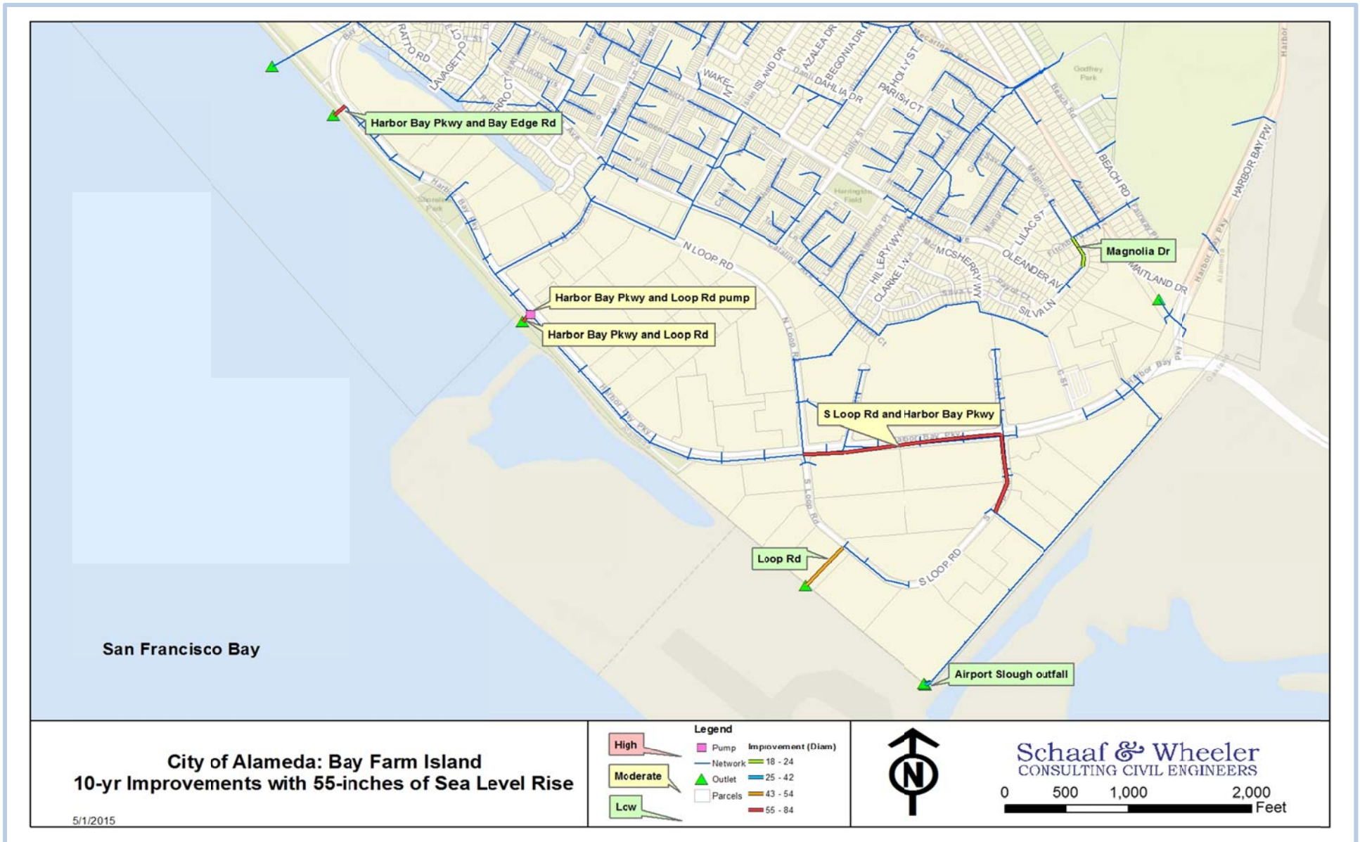
Figure 19: BFI South 10-Yr SLR Improvements
