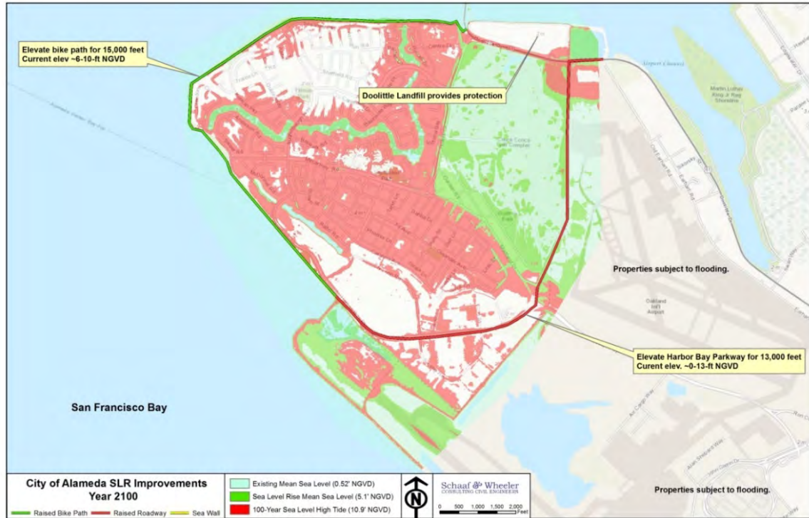
Figure 10 – Bay Farm Island Overland Improvements, 100-Year-Tide with 55 Inches of Sea Level Rise
