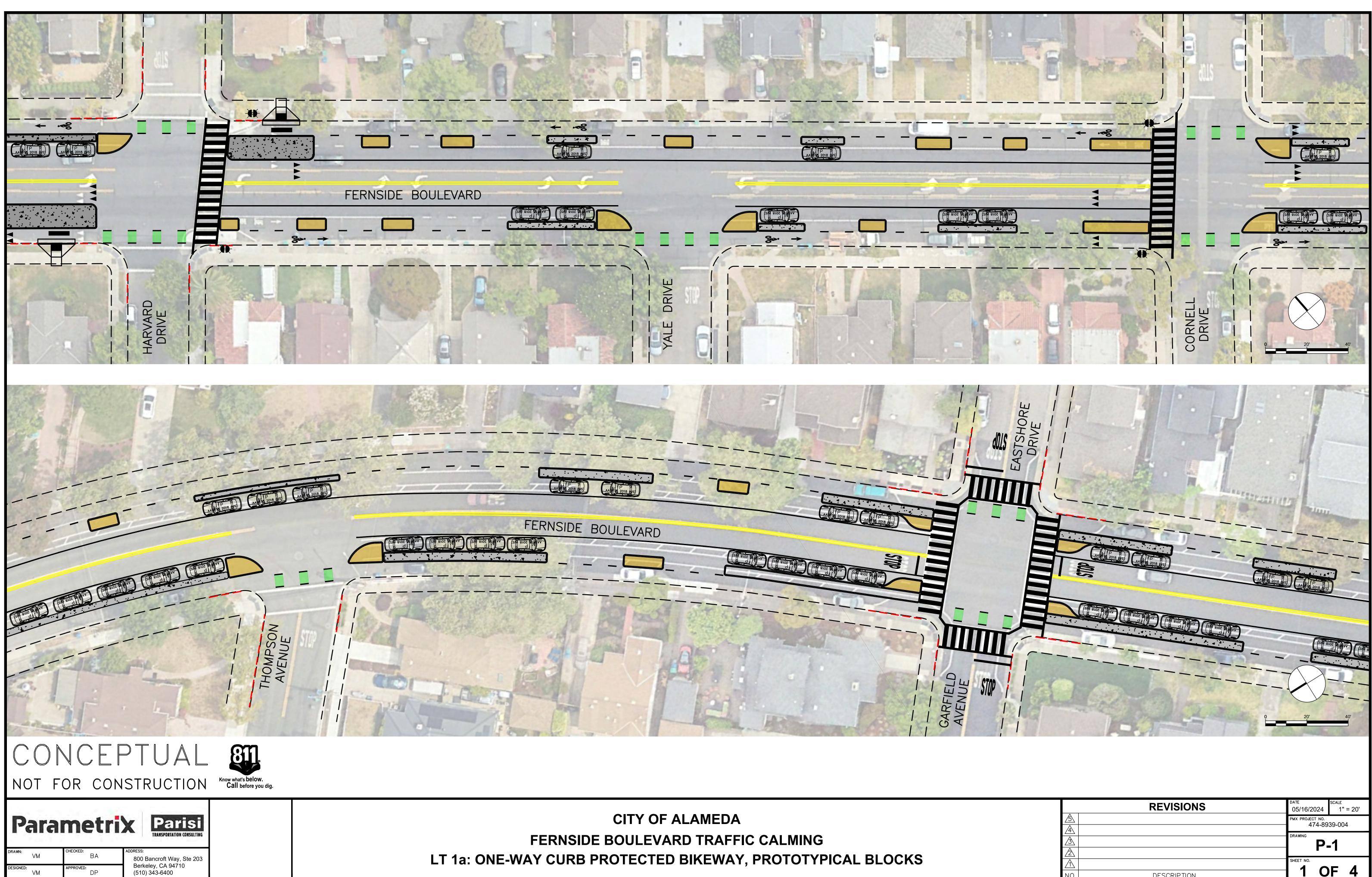
LT 1a: ONE-WAY CURB PROTECTED BIKEWAY, PROTOTYPICAL BLOCKS
