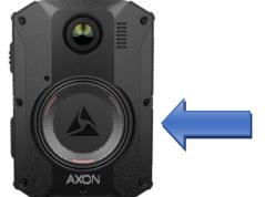
To begin recording, double-press the Event button. To stop recording, hold down the Event button for three seconds.
