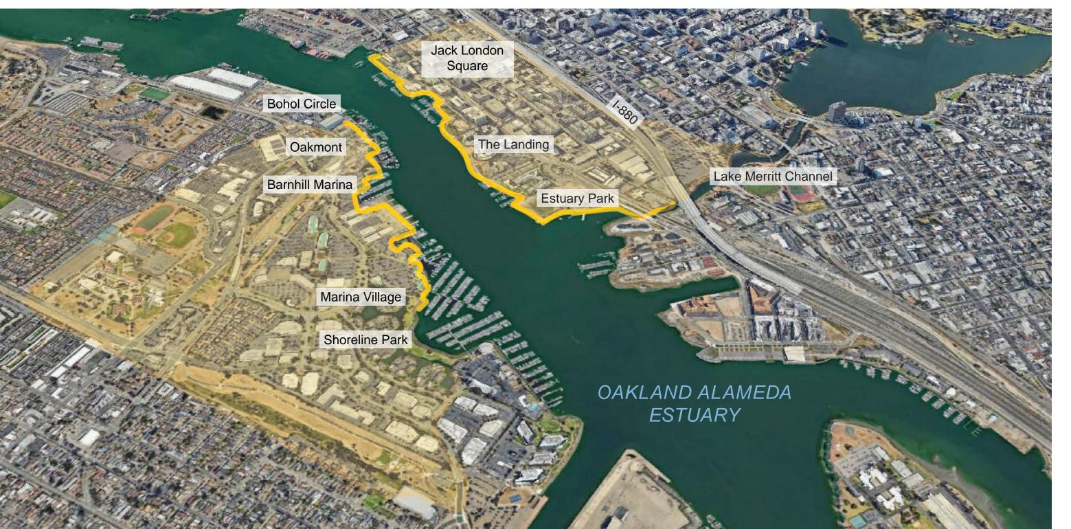
The **Oakland Alameda** Estuary Project is a near-term sea level rise adaptation design concept to address increased coastal, stormwater, and groundwater flooding for up to two feet of sea level rise over the coming decades. The project will include strategies to elevate and adapt low-lying areas of the shoreline combined with green infrastructure such as rain gardens and storm drainage improvements.
