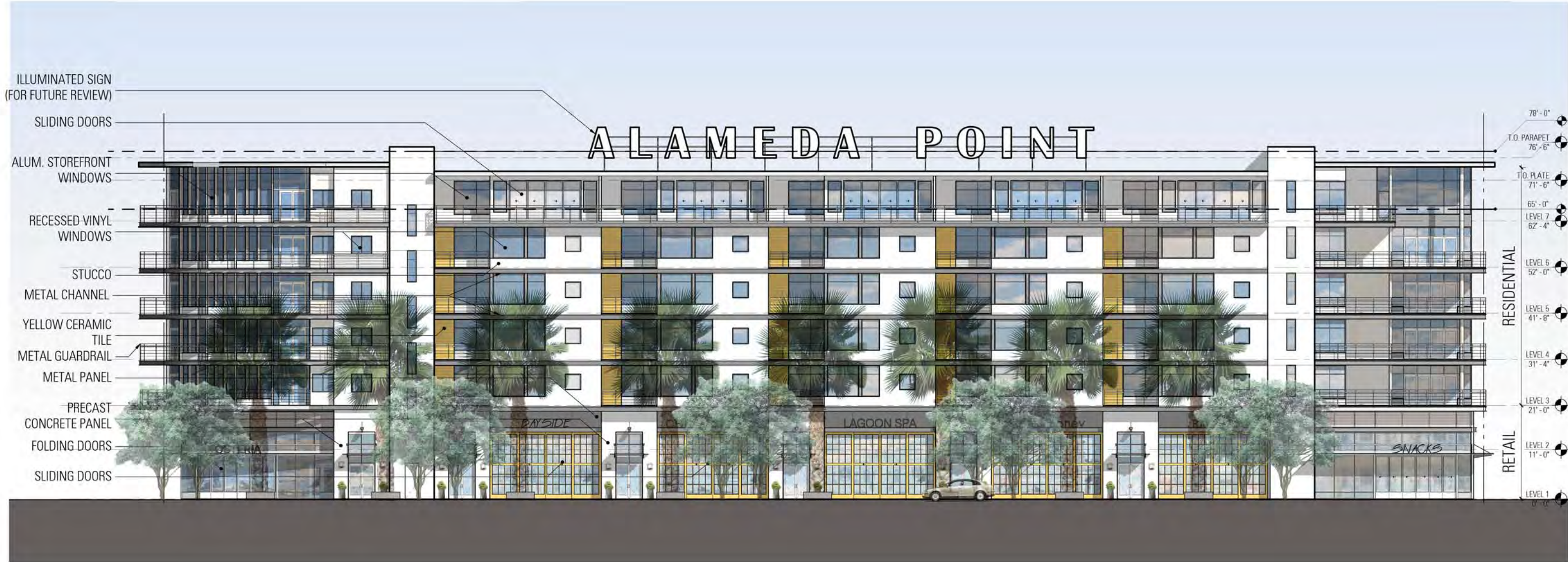
EXTERIOR ELEVATION - SOUTH
