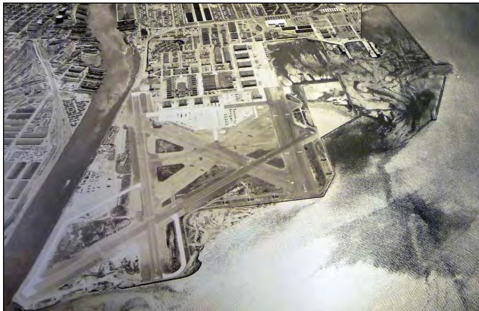
Photograph 31: 1954 aerial photograph showing the expansion of NAS Alameda runway system. Remaining portions of the World War II-era runways can be seen in the middle of the field. 134
