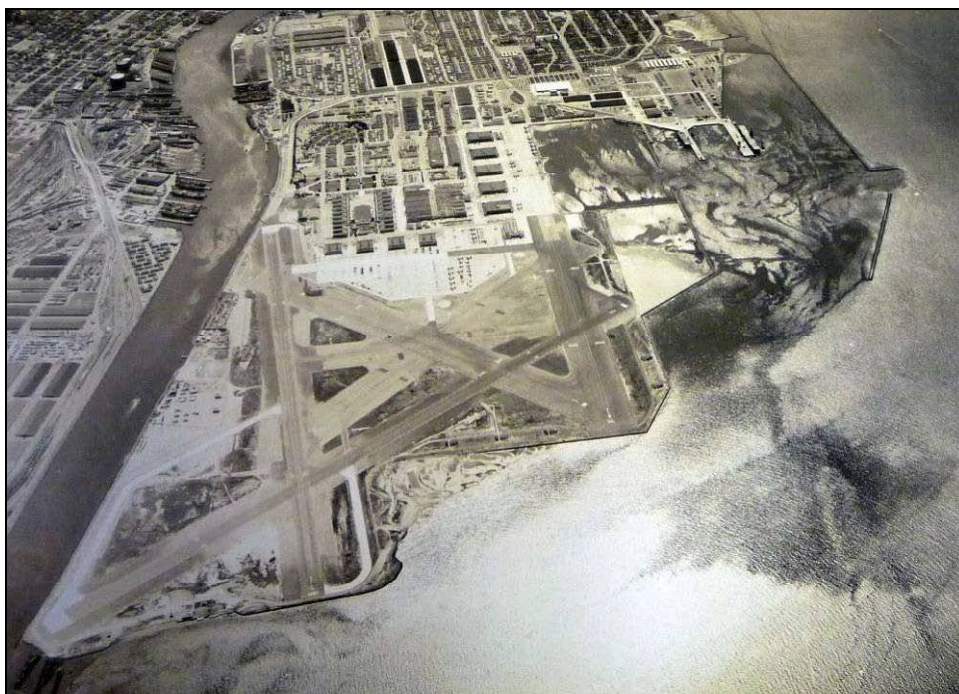
Photograph 56: 1954 aerial photograph showing the expansion of NAS Alameda runway system. Elements of the World War II-era runways can be seen in the middle of the field. 175
